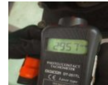
Figure 21. Check RPM Speed jockey pump
