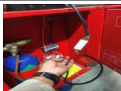
Figure 7. Function test pressure switch
